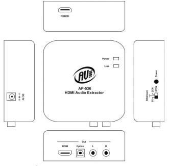
Connect the HDMI output from the source equipment to the HDMI In connector on the AP-536. Next, connect the AP-536's Optical or L and R outputs to the destination audio equipment. Optionally, connect the HDMI Out to an HDMI display device.
