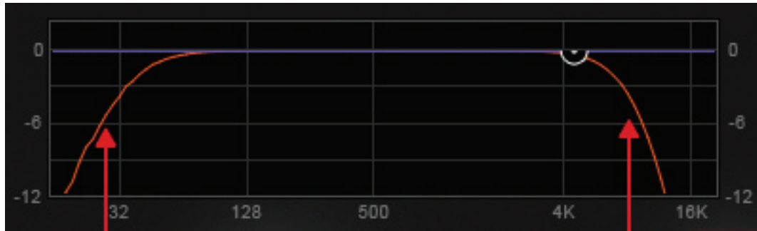
Comp's HP & LP Filters in Orange
