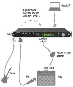
Figure 4-4: Recording guitar for re-amping.
