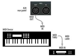
Figure 4-6: Connecting additional devices with MIDI THRU ports
