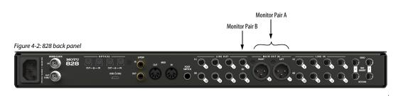
• Quarter-inch line outputs are not cross-coupled. Therefore, when connecting them to an unbalanced input, use a TRS plug with the ring disconnected. Not floating the negative terminal will short it to the sleeve ground and cause distortion.
