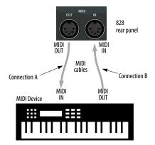
Figure 4-5: Connecting a MIDI device to the 828.
