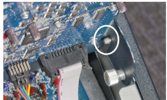
Figure 10. Correct alignment of Top Panel slot and pivot post
