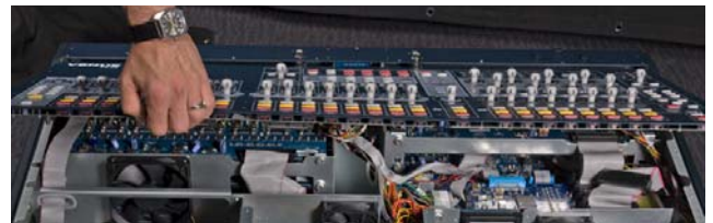
Figure 9. Lifting the Top Panel to vertical
