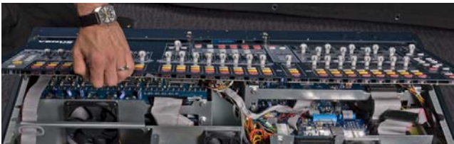
Figure 2. Lifting the Top Panel to vertical
