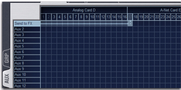
Assigning an Aux output to an A-Net Card in the Patchbay Outputs page
