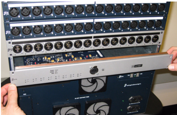
Installing an A-Net Card in Mix Rack
