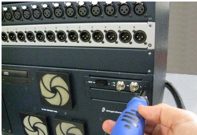
Installing the MADI card in the Mix Rack
