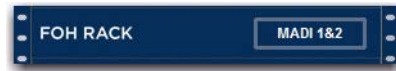
Two MADI cards indicated in the FOH Rack icon in the Devices page
