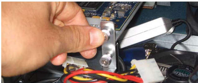
Tightening the captive thumbscrew
