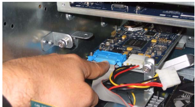
Attaching the ribbon cable to the MADI card
