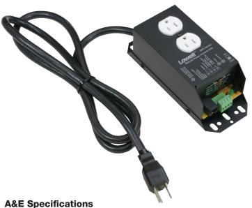
The device for remotely controlling AC power shall be Lowell Model No. RPC-15-SCD-RJ, which shall include a power supply and relay housed in a 7.5"L x 3.25"W x 2.75" steel chassis with black powder epoxy finish. The unit shall include one duplex outlet with 15A power rating and six ft. cord with NEMA 5-15P plug termination and basic surge protection up to 20,000A.
