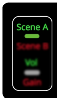
Figure 2: Scene A must be the active Scene on the PlayAUDIO12 to arm the unit for Automatic Failover
