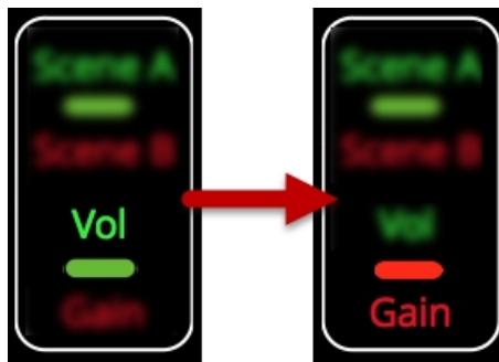
Figure 7: Press once to toggle between Volume display and Gain display modes.
