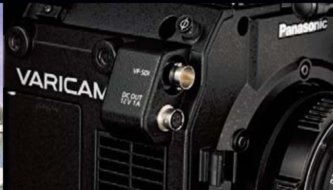
EVF Connections with HD SDI and DC Power
