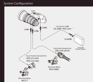
\*Connection cable for external power source is necessary when the power source (over 10V, 1A) car supplied from a camera.
