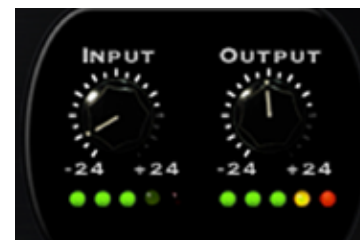
Figure 3: Output LED indicating maximum signal level
