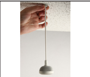
Fig J. Position the microphone by turning the cable as necessary and gently turn the nut clockwise to secure (1 to 2 turns). Do not over tighten.
