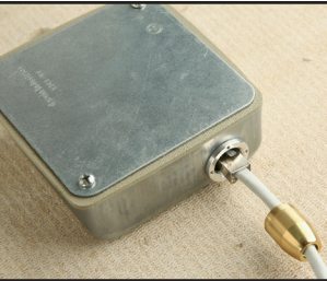
Fig G. Fasten the lid 3 on top of the junction box. Insert RJ45/ Cat cable into JBM3 receptacle. (See back page for installing seismic cable)
