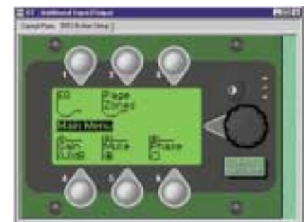
Programming can be totally checked off-line on the PC with the powerful 'simulate' mode.
