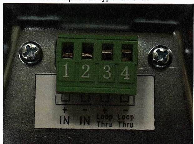
Fig. 32. The view of a plastic connection terminal used in loudspeakers CVS series
