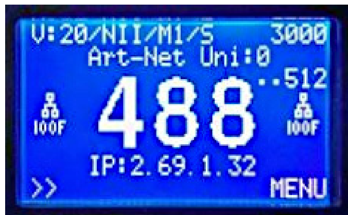
Figure 3. Display, Art-Net / sACN networks
