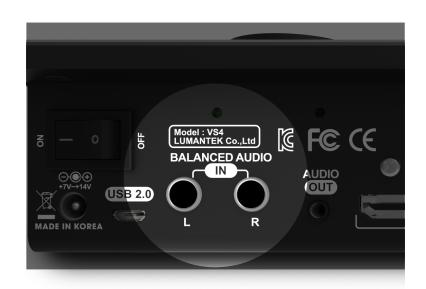
Stereo Balanced Audio input can be mixed with audio sources from 3G-SDI and HDMI video. Audio embedding and de-embedding supported.
