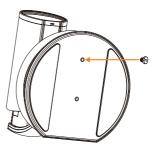
Secure the screw to the bottom of camera.
