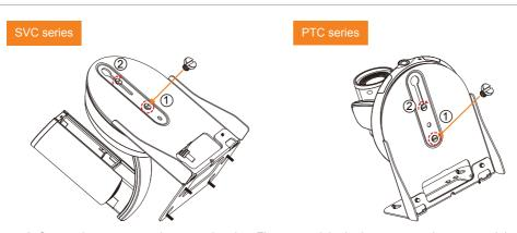
8. Secure the camera on the mount bracket. First, screw tight the lower screw, then, screw tight the upper screw.
