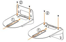
3. Asssemble the two mount plates and make sure the two mount plates are jammed. Next, secure two mount plates with screws.
