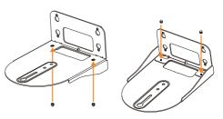
4. Install the nuts on the screws.
