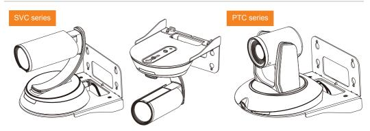
Complete.[Note] The PTC series camera doesn't support to mount in upside dowon position.
