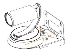
7. Connect the necessary cables to the camera. Then, slide the camera in the end.
