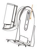
Slide the camera into the mount bracket. Don't slide camera in the end, before installing the cables to the camera.
