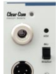
KB-211GM (detail showing mic connector and mic/headset switch)
