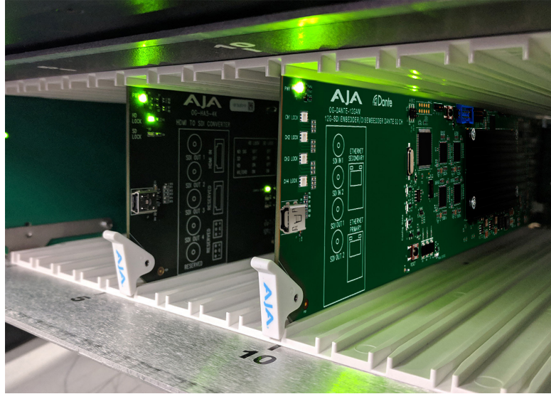
Figure 9. The white plastic tab for the card on the right is now upright. Both cards are shown fully inserted.
