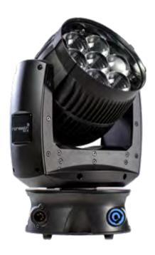
The small size of the impression X4 S does not give way to any compromise, as the heart of the impression X4S features seven high powered RGBW LED's, each rated at 15 Watts, that combine to give a homogeneous output across its entire beam range. Its 7° to 50° zoom offers the flexibility of a tight beam mode thru to a smooth edged wash light.
