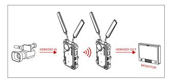
Note: The transmitter can be equipped with mushroom antenna. When there is a large height difference between the transmitter and receiver, it is recommended to use Hollyland mushroom antenna at the transmitter to improve the stability of wireless transmission.
