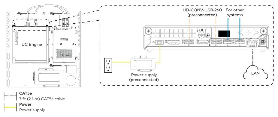
3. Connect displays to the UC Engine.
