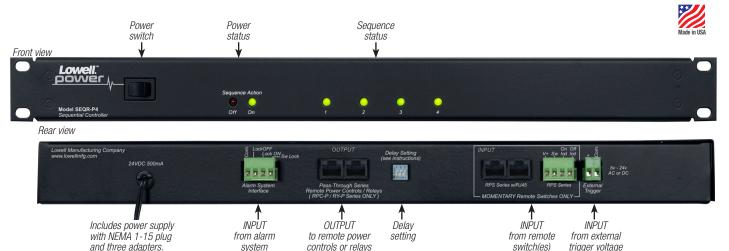
**DESCRIPTION:** This low voltage power sequencer with pass-through RJ45 jacks for quick connections works with compatible remote power controls (RPC-P Series) and relays (RY-P Series) to provide time-delayed activation and deactivation of AC powered equipment at remote locations.
