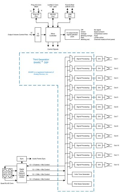
External control, the user interface and signal flow are shown in the diagram at left. Multiple DM Series units interconnected in a system pass control information and audio signals via the DANI™ bus (Digital Audio Network Interface) as shown in the diagram.
