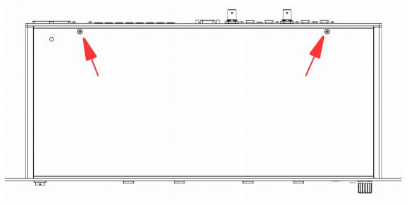
■ Flip the multiverter to detach the top cover. Disconnect the cover's ground connection at the base.
