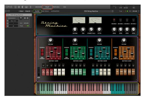
Adjust parameters in the **GLOBAL CONTROLS** AREA to finalize the master stereo output of an instrument by using volume, pan, stereo field, filter, and reverb controls.
