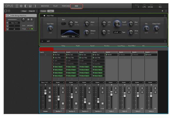
The 4 Sub Mixer channels provide independent outputs for Instrument Sections 1-4, enabling unique effects settings for each. The Pan Tool and Auto Filter effects are enabled across all 4 sections by default, and the ADT and Ensemble effects can be turned on here in the Mix page, or in the Play page by clicking the respective 'Chorus' and 'Ens Chorus' buttons.
