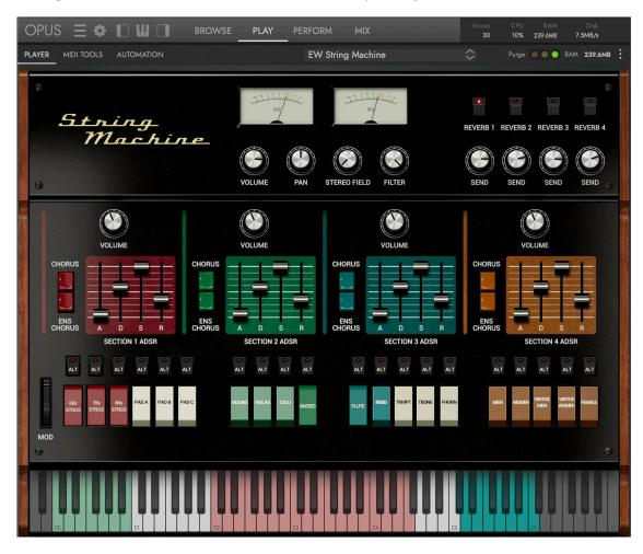
String Machine's user interface is inspired by the design of vintage string machine synthesizers, from the chunky instrument switches adorned along the front panel, to the glide of envelope sliders, and the tactile 'feel' of push buttons.
