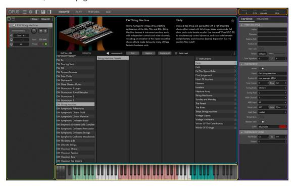
The **INSTRUMENT RACK** AREA populates with loaded instruments, and includes basic controls for volume, pan, solo / mute, and more. Further details are just below.
