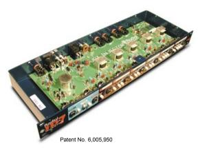
The Radial JD7 Injector is a guitar signal distribution system that allows control over as many as seven amplifiers from one guitar. The JD7 is optimized to ensure the true natural tone and feel of the guitar is maintained while eliminating noise caused by ground loops.
