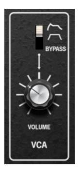
**Volume and modulation controls**- The VCA section controls overall amplitude (volume). The slides switch chooses between amplitude control via the ADSR envelope generator, the AR envelope generator, or *Bypass* mode.
