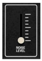
**Noise Level**- Sets the volume level of The Cat's white noise generator. For those of you hoisting clipboards, white noise is a random signal in which all frequencies across the frequency spectrum are represented equally.
