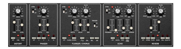
The Cat includes five simultaneous effects: Distortion, Phaser, Flanger/Chorus, Delay, and Reverb. These can be used in any combination.
