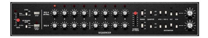
Cherry Audio's Octave Cat includes a dual-channel, eight-step sequencer. The sequencer CV's can be independently assigned not only to oscillator pitches, but also to filter cutoff and VCA amplitude.
