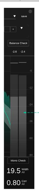
The output meter displays the current peak and RMS value for each channel. The small number above the meter shows the current RMS value.
