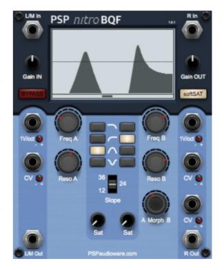
The Resonance can also be controlled with CV and the CV signal can be further modified with the CV trim knob below.
