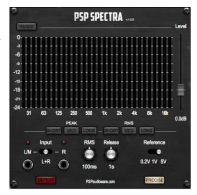
The **Input** toggle changes the displayed signal between the Left (L/M), Left and Right (L+R), and Right (R) channels. For Left and Right mode, both input jacks must be used.
