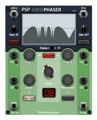
The **Depth** knob adjusts the depth of the phaser effect. This can be modified using CV, with the cv being further adjustable with the cv trim knob.
