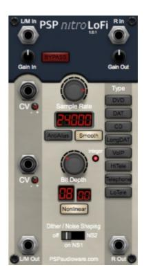
The Bit Depth can be modified with CV, with the CV being further adjustable with the CV trim knob.
