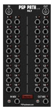
The **Output** side features 16 monophonic CV inputs which can accept mono CV sources from the Input side of the matrix, or from external sources.
