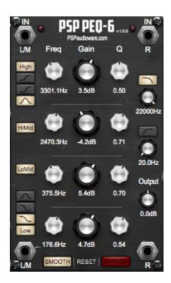
The **Lowpass** button is used to enable the Lowpass Filter, with the Frequency set by the knob below.
