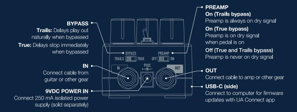
Power Supply Isolated 9VDC, center-negative, 250 mA minimum,
