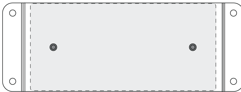
Align the holes as shown for securing a single device in the single-unit mounting tray
