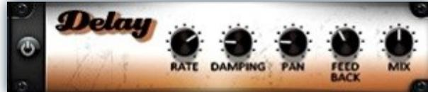
**Feedback** - This knob controls the feedback of the delay effect. High values can cause an endless loop.
