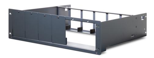
The Bluesound Professional RM160 is a rackmount system allowing up to 6 x B160S network streaming stereo amplifiers to be mounted in a 3U space in a 19" rack. The B160 modules slot in from the front and are secured by a front panel screw, allowing for swift replacement when required. B160S units are supported front and back.
