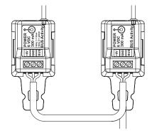
**Caution**: The PXE-EMIT-REL2 is for low voltage control only and **under no circumstances should it be connected to high voltage**.
