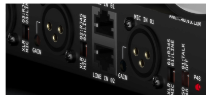
StudioHub+ RJ45 connectors for lines. XLR connectors for mics.
