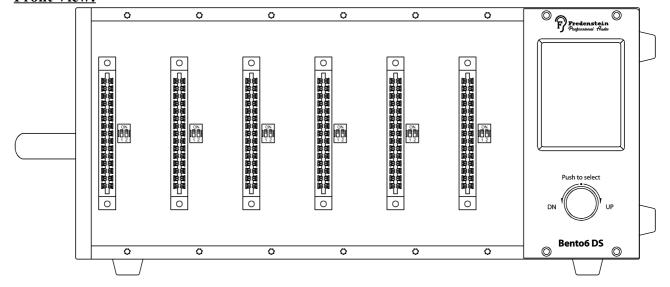
If certain non-Fredenstein modules are used, which bridge several pins on the connector and connected the contacts on the top and button side, the double switches, located directly besides the slot connectors, can both be turned off (lower position) to avoid interference between the module and the digital interconnect. For Fredenstein modules, both need to be in the ON (upper) position.
