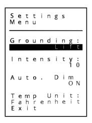
In case of severe ground loops you might engage the ground-lift to alleviate such problems. But it is always recommended to resolve the grounding problems at their source and keep the ground-lift switch disengaged (OFF). Select Lift and push the wheel to toggle between off and on.
