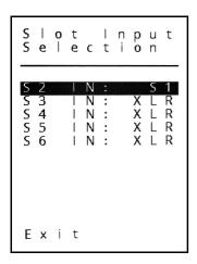
In the Slot Input menu the input signal for slots 2 to 6 can be selected. (Slot 1 always gets its input signal directly from the XLR connector located on the back-panel). By turning the wheel the desired slot can be selected and by pushing the wheel the value toggles between XLR for the slots input XLR connector or the output of the slot to its left. Selecting Exit will show the Setup Menu again.
