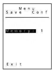
Ten different setups can be stored. By selecting Memory and push the wheel and the number of the setup is highlighted, turn the wheel to the number you want to use, then press the wheel to store the configuration. Selecting Exit and pushing the wheel will show the Setup Menu again.
