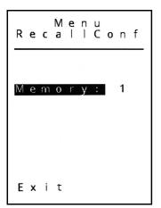
To recall stored select Memory and push the wheel and the number of the setup is highlighted, turn the wheel to the number you want to use, then press the wheel to recall this configuration. Selecting Exit and pushing the wheel will show the Setup Menu again.
