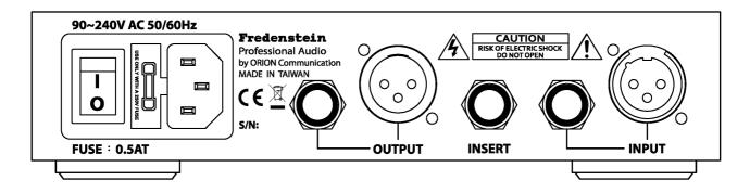
Please connect your microphone input and the output first to the XLR or TRS connectors located on the back panel. Connect the mains cable to the V.A.S. MicPre and then to a grounded mains outlet. The power ON/OFF switch is located on the back panel near the power cable connector (IEC). After the unit is powered on, the PWR indicator on the front panel will be illuminated.
