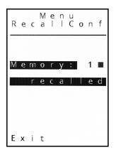
To recall stored configurations, select Memory and push the wheel and the number of the setup is highlighted, turn the wheel to the number you want to use, then press the wheel to recall this configuration. A square mark behind the number indicates that this memory location holds a valid configuration and can be recalled. The "recalled" message appears after a successful read of the nonvolatile memory. Selecting Exit and pushing the wheel will show the Setup Menu again.
