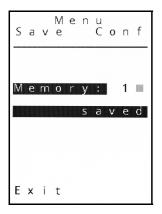
Ten different setups can be stored. By selecting Memory and push the wheel and the number of the setup is highlighted, turn the wheel to the number you want to use, then press the wheel to store the configuration. A square mark behind the number indicates that this memory location is already used, but it can be overwritten. The "saved" message appears after a successful write to the non-volatile memory. Selecting Exit and pushing the wheel will show the Setup Menu again.
