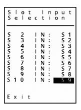
In the Slot Input menu the input signal for slots 2 to 9 can be selected. (Slot 1 always gets its input signal directly from the XLR connector located on the back-panel). By turning the wheel the desired slot can be selected and by pushing the wheel the value toggles between XLR for the slot input XLR connector or the output of the slot to its left. Selecting Exit will show the Setup Menu again.
