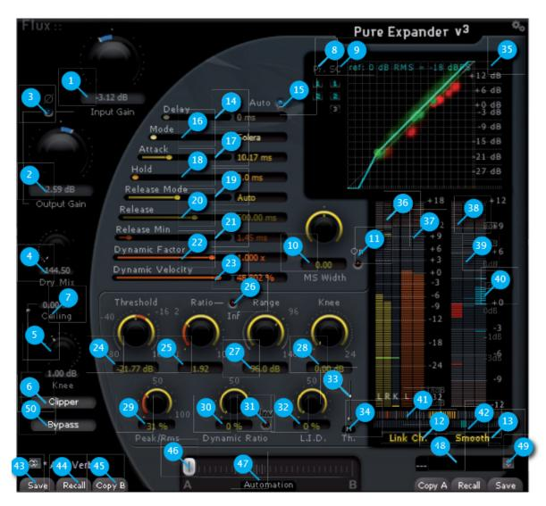
Pure Expander is the expander section of the Solera. An expander is used to automatically reduce the gain below the Threshold. The exclusive Dynamic Ratio algorithm developed by Flux:: allows you to remove unwanted noises or reverberation without adding a processed character to your sound. Pure Expander produces a wide range of expansion process from subtle expansions to hard noise-gate.
