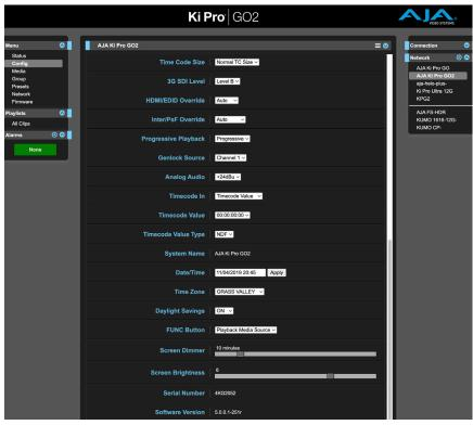
The Config screen provides access to the Config menu parameters (see "CONFIG Menu Parameters" on page 29), except Network configuration settings are available on the Web UI Network panel (see "Network Panel" on page 51).
