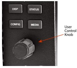
When an active configuration menu is displayed, pressing and holding the knob will restore that menu's factory default setting.
