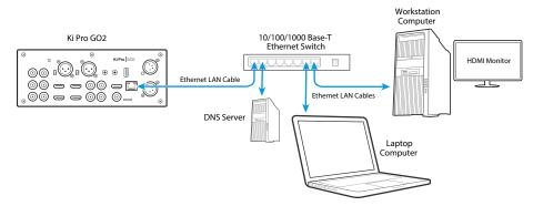
LANs may be divided into zones, and devices on a LAN may have dynamically assigned (DHCP) IP addresses, or fixed (static) IP addresses. Before connecting Ki Pro GO2 to the LAN, talk to your network administrators to find out how they want it connected (DHCP or Static IP). If your LAN requires static IP addresses, also ask your IT administrator for the Subnet Mask and Default Gateway IP addresses (your LAN's Internet router).
