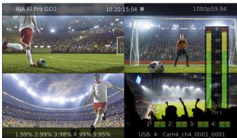
Figure 5. Audio Meters Front Panel Display Example
