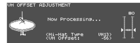
The "VH Offset" parameter is set automatically (approx. 3 seconds). The [TRIGGER] button stops flashing and remains lit.
