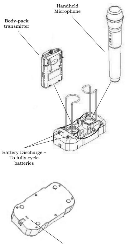
Specifications: Dual Slot Charger: Charges two IRH-30 handheld microphones and two IRB-30 body-pack transmitter. Discharging: .. Two buttons (yellow) to fully cycle batteries Charging Buzzer: .. ON/OFF switch, buzz's when batteries are fully charged Charging Speed: .. 400mA / hour
