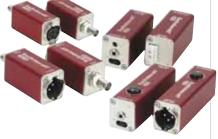
terminal block line-level output with pad and lift switches. The 366R is an AES/EBU adapter which converts female XLR  $1\overline{10}$ ohm to BNC 75ohm. The 367R is an AES/EBU adapter which converts BNC 75ohm to male XLR 110ohm.
