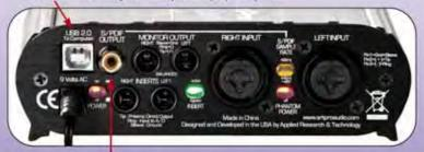
S/PDIF output for expanding inputs on digital workstations and computer interfaces
