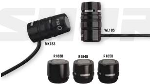
SHURE MICROFLEX LAPEL MICS The Microflex lapel condenser mics feature high sensitivity, a frequency response of 50Hz-17kHz, interchangeable condenser cartridges (MX models), & a variety of low-visibility mounting options. MX models are terminated to XLR & include a belt-clip preamp. WL versions are terminated with TA4F connectors for Shure wireless systems.
